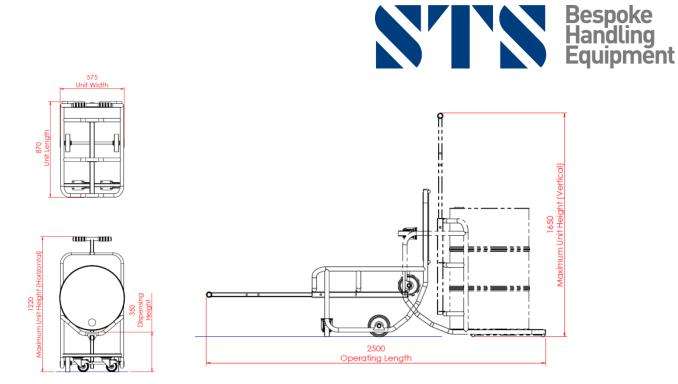
The below image shows the easy procedure of loading the DCR01 ready to rotate and dispense a 200 litre drum.
